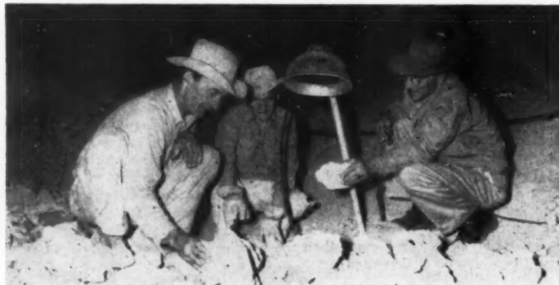
Foreman Joe Courson, miner Art Byers, and manager A. C. “Al” Lambert examine freshly broken scheelite ore under the powerful floodlight of a Model S-61 Mineralight.
